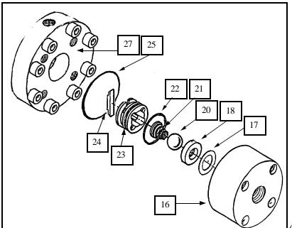
Remove the four bolts (ref# and pull intake endcap (ref# 16), from the pump. The endcap should separate from the material head (ref# 27), with the ball guide (ref# 23) attached. If the ball guide remains in the material head, pry out with a screw driver.
